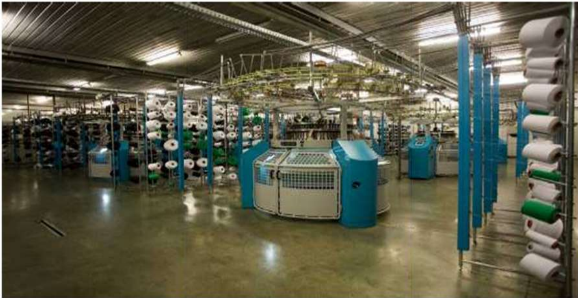
Figure 4.2.7. Circular Knitting machines in different gauges, at RECO Textile.
