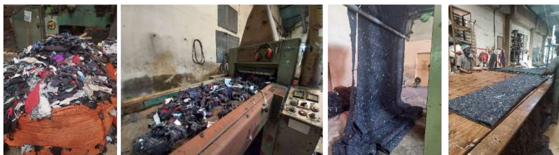
Fig. 4.1.6 Recycling of textile waste into non-woven rugs at Blanket Industries - Mombasa
